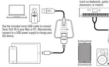
Use the included 14-pin to Lightning cable to connect Sonic Port VX to your iOS device
